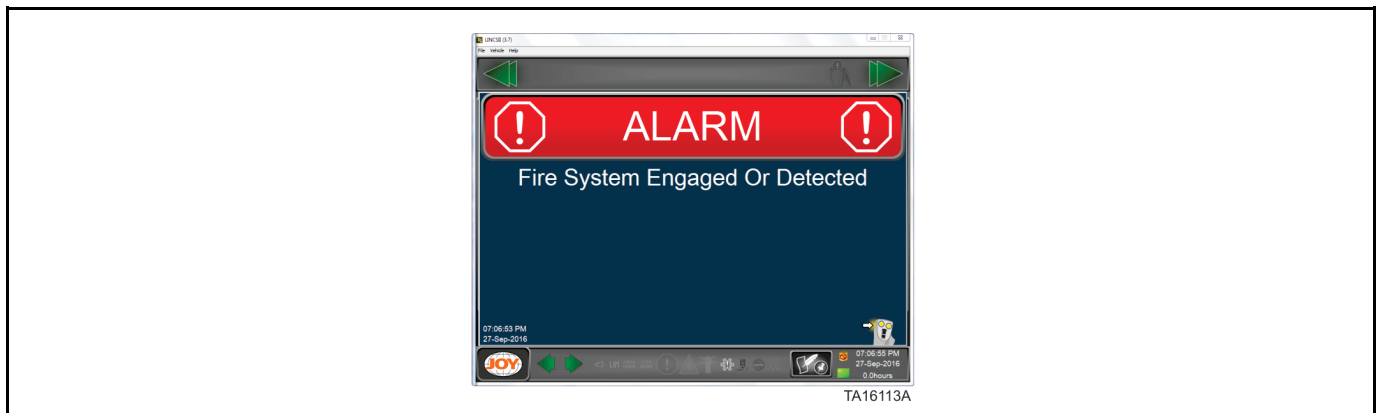
Figure 17: Fire suppression system engaged or detected red alarm screen
